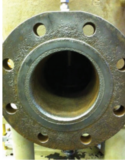
13, 14. Gas control valves can suffer severe corrosion (left) as evidenced by 35-mil loss of metal in some areas (right)
