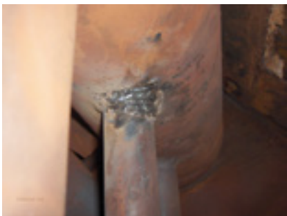
18-19. Puddling weld material is not a proper repair (left); professional weld is at right
