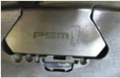
4. PSM's R0 retention plug replaces the biscuit familiar to many users
