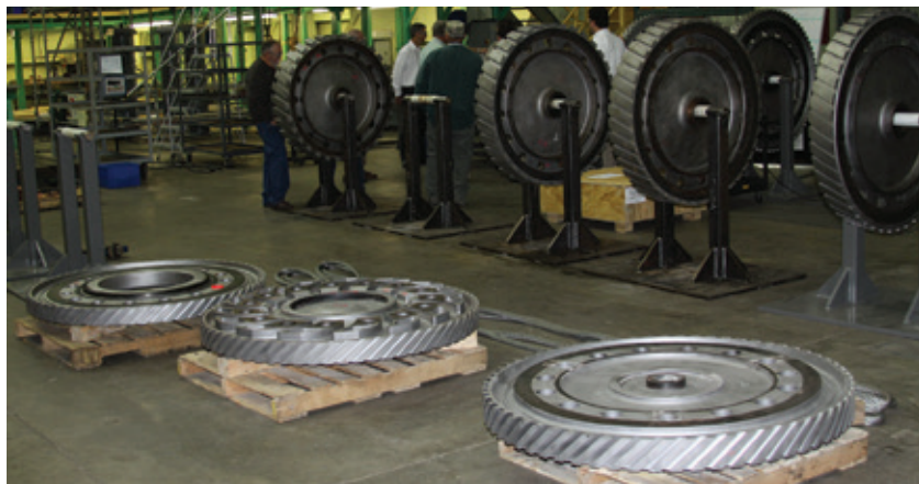
C. Compressor section was disassembled after blades were removed
