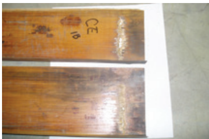
7, 8. Slot insulation burn-through (left) and cracking of flex leads resulted from a field ground fault
