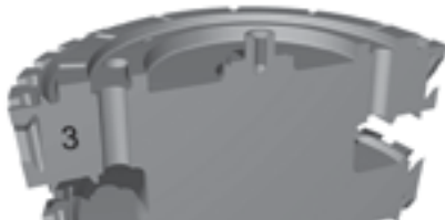
7. Pilot incorporated into the Stage 3 wheel on the LP stub has an internal thread, used for lifting
