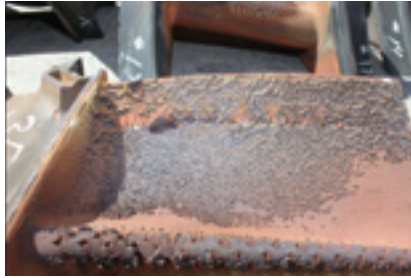
1. Iron and other contaminants in wetted-media evap cooling water stuck to turbine blades (buckets)
