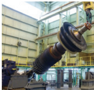
A. 7FA rotor is received at Alstom shop for repairs
