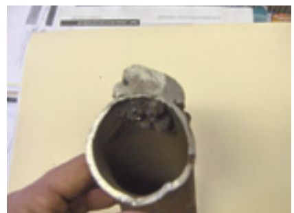
2, 3. Ugly “repair” of U-bend passed hydro (left); section through the weld area is at right
