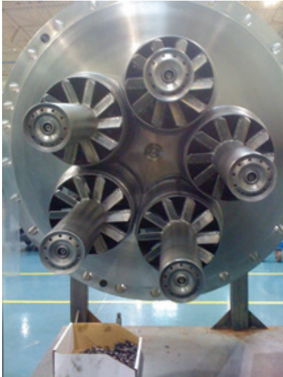
4. DLN2 was introduced on the 7FA (model 7221) as a 25-ppm-NO x combustion system. Note the ring of five nozzles, no center nozzle. This system was replaced by the DLN2+ before the millennium
