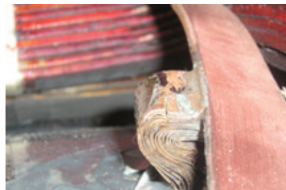
7, 8. Slot insulation burn-through (left) and cracking of flex leads resulted from a field ground fault
