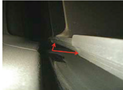
21. Inspectors check for platform wear on the trailing edges of S1 vanes.
