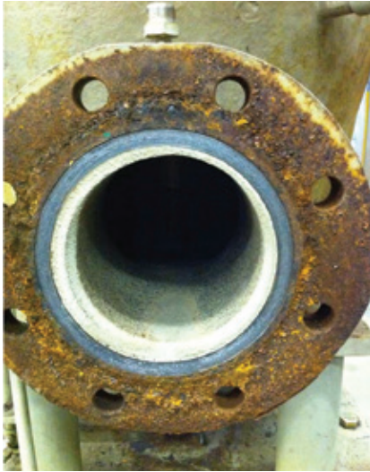
13, 14. Gas control valves can suffer severe corrosion (left) as evidenced by 35-mil loss of metal in some areas (right)
