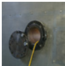
Penetrations on enclosures eliminate the need to run lines, cords, and leads through doorways. Walter M Higgins Generating Station
