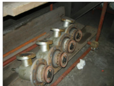
1. The road to DLN2 began with a single-nozzle conventional combustor—simple, inexpensive, robust. Water or steam was used for NO x suppression
