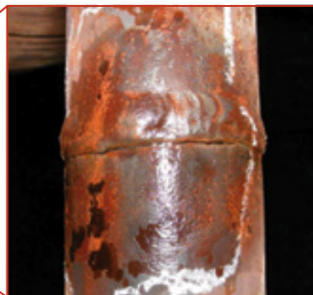
3. Drains that collide with the floor liner or casing often suffer stress-induced cracking
