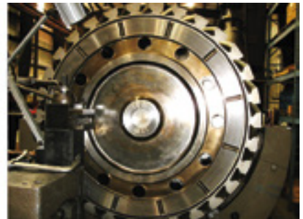
11. Insert was designed to take the place of the pilot, which is used only during the rotor assembly process, and installed in the wheel
