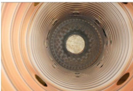
1. The road to DLN2 began with a single-nozzle conventional combustor—simple, inexpensive, robust. Water or steam was used for NO x suppression
