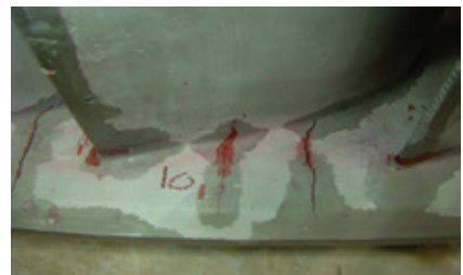
9. Cracking of first-stage nozzle to the degree shown suggests replacement, not repair
