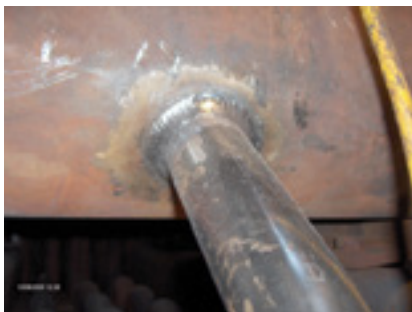
18-19. Puddling weld material is not a proper repair (left); professional weld is at right
