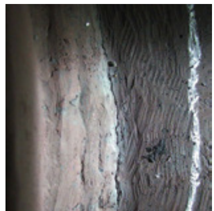
5. Spray nozzle assembly in probe-type desuperheater is susceptible to thermal fatigue damage
