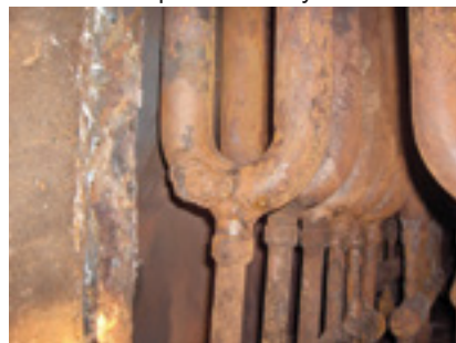
2, 3. Ugly “repair” of U-bend passed hydro (left); section through the weld area is at right
