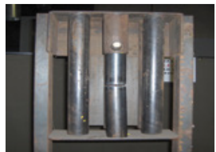
4, 5. Good weld on back side of tube was made using mirror; mirror test jig for practicing welds and for qualifying welders is at right
