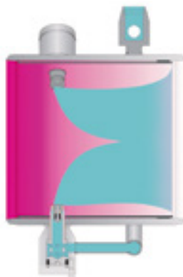
10. Fixed-orifice nozzles are not suitable for use in combined cycles in daily-start service
