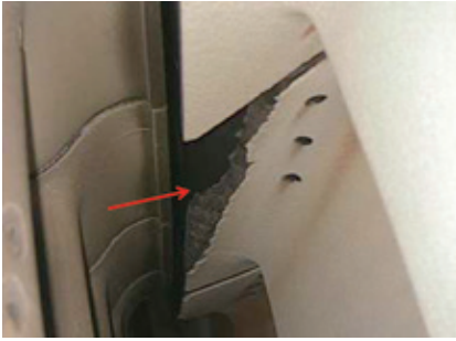
17. Erosion at the base of vane segments is found occasionally
