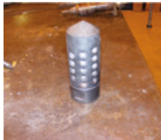
10. Fixed-orifice nozzles are not suitable for use in combined cycles in daily-start service
