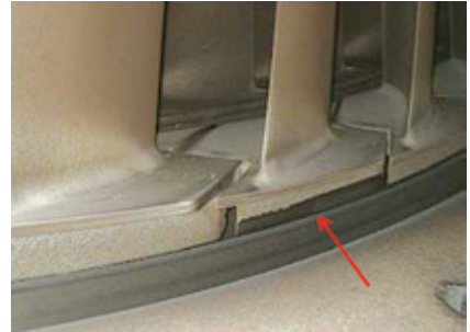
22. Rotor-blade tip shroud rub sometimes is identified in R3 and R4 of the power turbine
