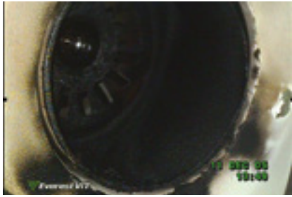
3. Coke accumulation on a primary nozzle after a four-hour run on distillate and oil shutdown
