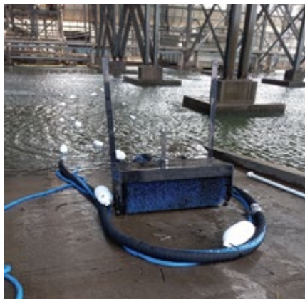
2. Drive mechanism for the remote cleaning device is at the left, the brush doing the work is at the center, and the controllers regulating the activity are at the right
