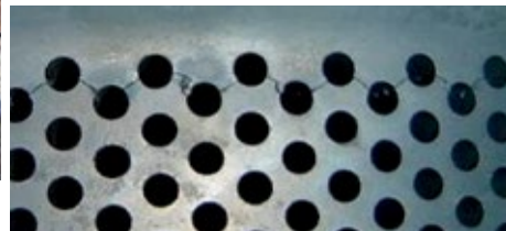
Valve trim damage
