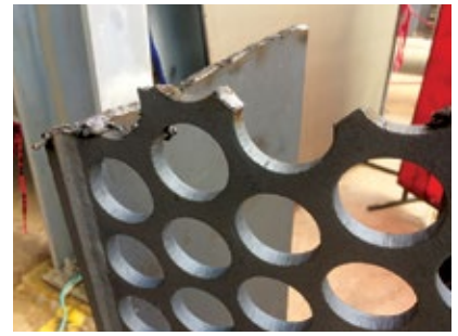
4. Perforated plates help ensure GT exhaust gases are evenly distributed when they reach the HRSG's heating surface, burners, and catalyst
