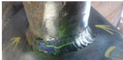
Branch-to-nozzle weld crack
