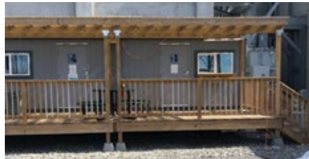
9. A mobile LOTO trailer with modular deck was provided for outages. It is equipped with power, heat/AC, domain network cables for the LOTO officer's computer, plus shelving and organization for all LOTO job boxes. The trailer and deck can be moved easily to provide convenient access to the work
