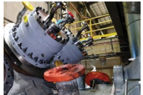
2. Combustor-within-a-combustor design enables advanced flame staging. Combustor's low pressure drop benefits heat rate, contributes to smaller footprint
