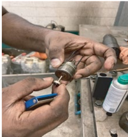
3, 4. In-house maintenance of fuel-oil injectors at Levant was highly successful
