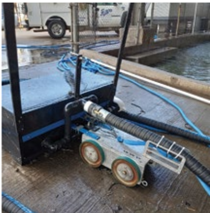
2. Drive mechanism for the remote cleaning device is at the left, the brush doing the work is at the center, and the controllers regulating the activity are at the right
