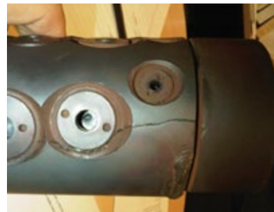
Cracked probe body
