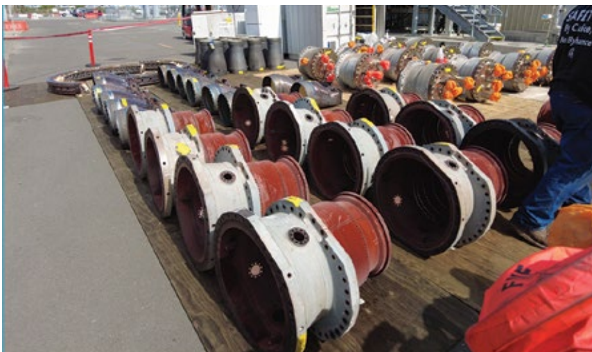
2. Damaged 7F.05 combustor hardware sits on the grounds of a highly cycled plant serving a grid characterized by a "canyon" dispatch curve in the spring
