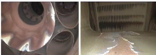
5, 6. Combustion coating loss and cracking (left) and transition-piece seal erosion (right) are two of several damage mechanisms identified in the 501G line of machines
