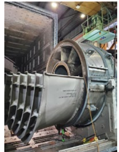
8. Upgraded 7EA-style split aft diffuser (left) is installed in shop (right)
