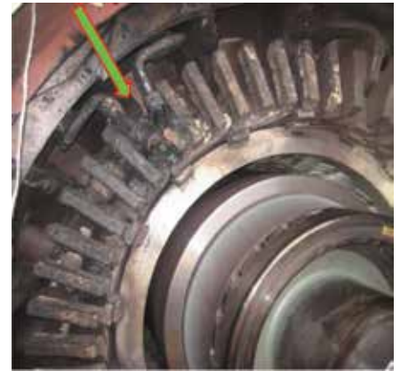
Sulzer. Rotor arrangement for a W501FD2 shows locations of problem areas noted in the company’s presentation discussing its repeatable repairs and solutions
