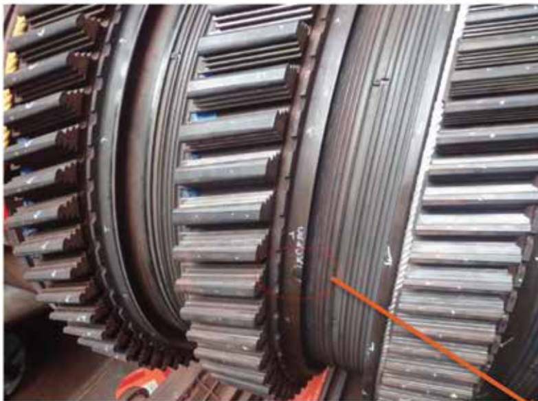
Crack found in Row 2 was excavated, then blended using a 5:1 ratio
