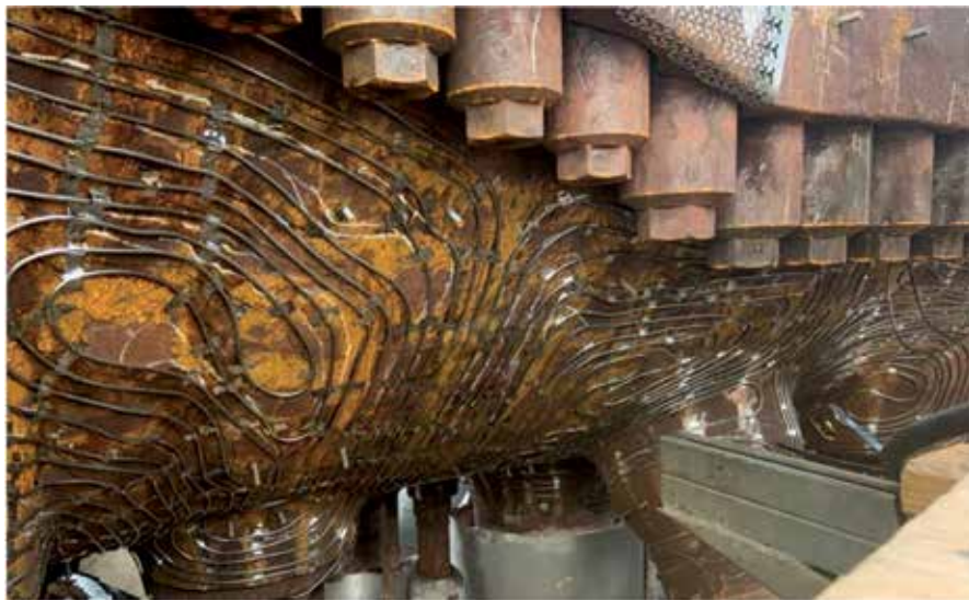
ARNOLD Group. Permanent placement of redundant sets of heating wires on the casing below the split line, plus the use of a heat-reflecting
