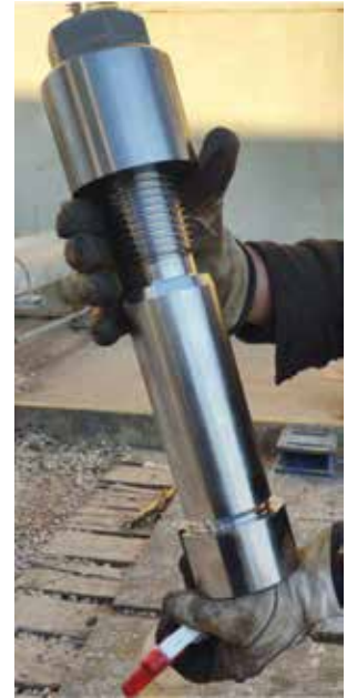
Use of Siemens-Energy’s upgraded hardware facilitates removal and replacement of generator coupling bolts, nuts
