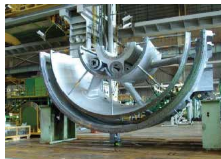
Doosan Turbomachinery Services. New exhaust cylinders (standard two-piece configuration) and exhaust manifolds in production enable in-kind replacement with DTS enhancements
