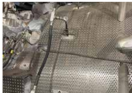
2. Thermocouples monitor average blade-path temperature
