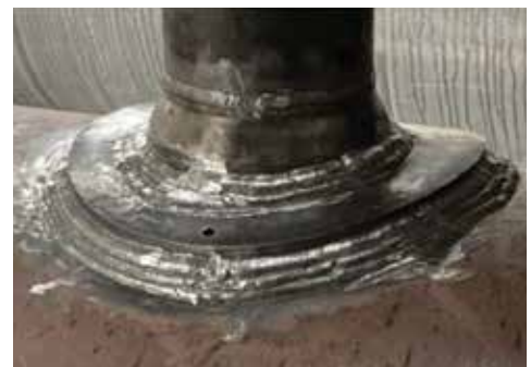
1. Nozzle welds may require reinforcement
