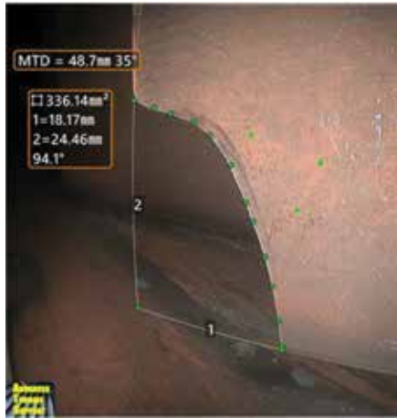
Advanced Turbine Support. In-situ blending mitigates the possibility of further damage, saves time and money by minimizing the extent of unit disassembly required
