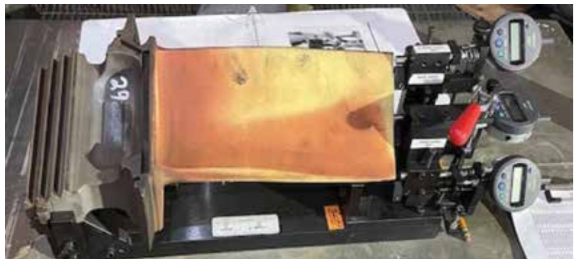
Field tipping of Row 1 blades was cited for dealing with rubs
