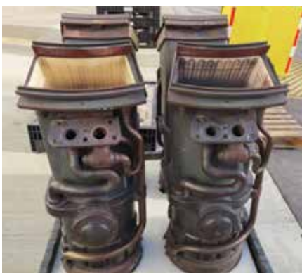
1. Steam piping is clearly visible on the transition pieces
