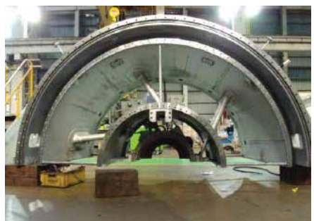
Doosan Turbomachinery Services. New exhaust cylinders (standard two-piece configuration) and exhaust manifolds in production enable in-kind replacement with DTS enhancements
