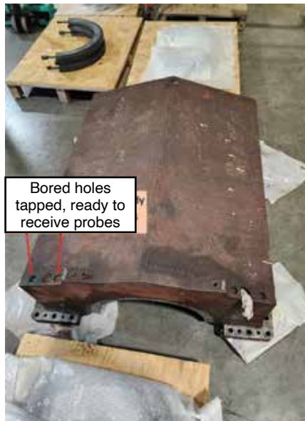
Bored holes for seismic probes as found after cover lift (left), holes tapped and ready to install seismic probes (center), locations of the original probes and additional probe (right)
