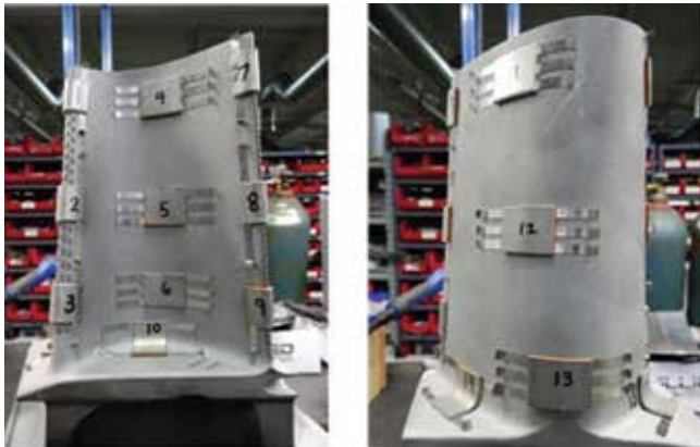
3. Use of tabs allow use of the same buckets in multiple trials
