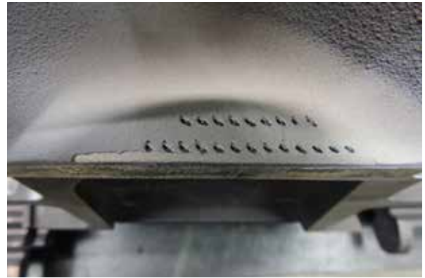
4. TBC top-coat spallation at this S1B's platform edge prior to installation
