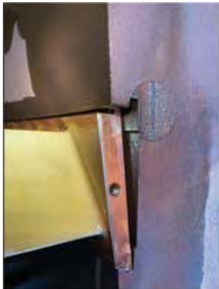
Hook-fit issues also were discovered on this M501F3
