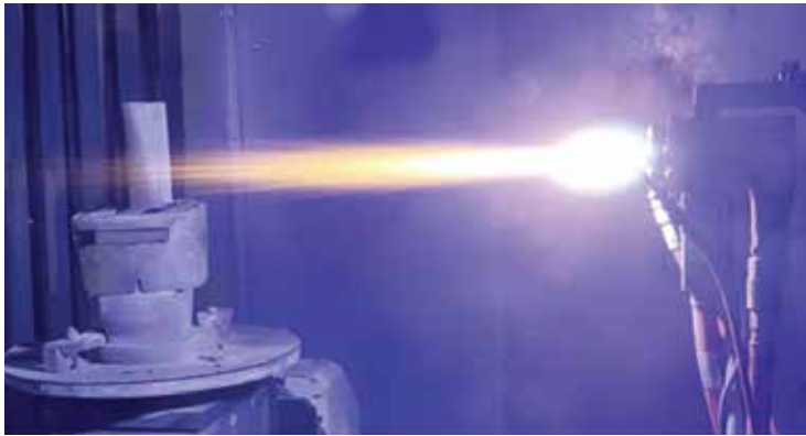
2. Air plasma spraying of a first-stage bucket
