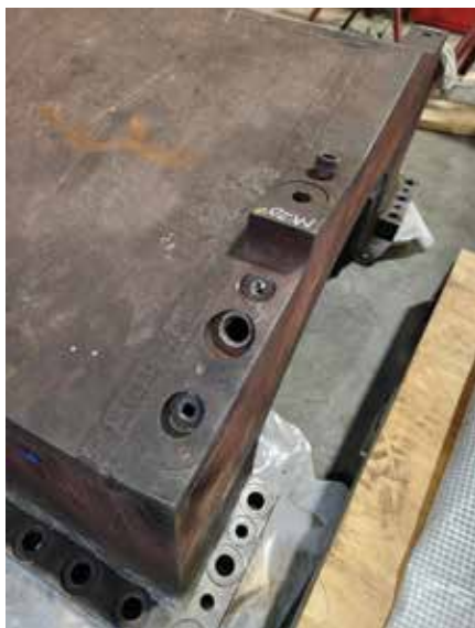
Bored holes for seismic probes as found after cover lift (left), holes tapped and ready to install seismic probes (center), locations of the original probes and additional probe (right)
