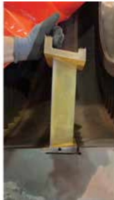
Hook-fit issues also were discovered on this M501F3
