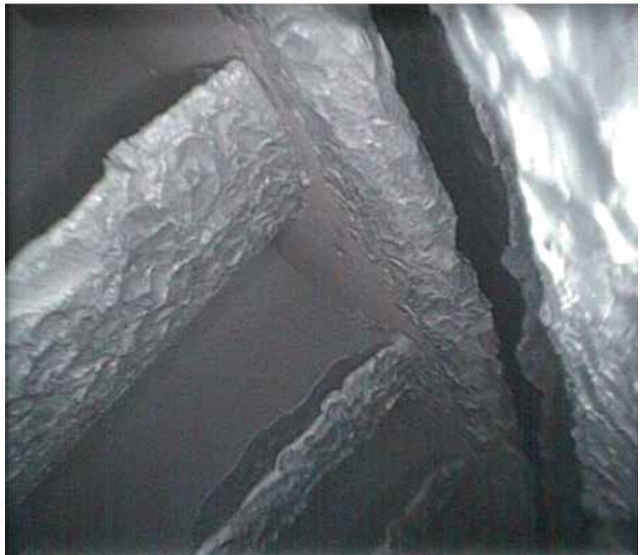
Damage to steam-turbine blades attributed to disbonded Stellite
