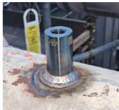
1. Nozzle welds may require reinforcement
