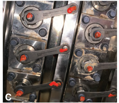
Effects of increased cycling on VSVs: (A) Black carbon “smoking” around the lever arm is a clear indication of wear and helps with all tubing and piping inspections as well. “If its smoking, its rubbing,” Clutts remarks. (B) VSVs not secured correctly and/or inspected will cause a stall. (C) Signs of contaminated water intrusions noted during VSV inspections
