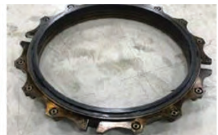
2. FT8 bearing issues like carbon seal wear can impact oil flow and cause scoring. Proposed solutions include seal replacements and material improvements to address vibration along with closely monitoring oil consumption and particulate
