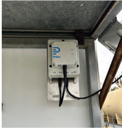
2. Communications link transmits data captured externally
