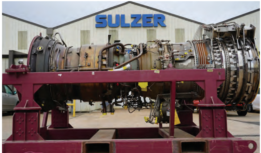
9. FT8 engine purchased by Sulzer for purposes of reverse engineering development starting with component repair, tooling design and fabrication, and eventually, new parts manufacturing
