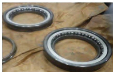
2. FT8 bearing issues like carbon seal wear can impact oil flow and cause scoring. Proposed solutions include seal replacements and material improvements to address vibration along with closely monitoring oil consumption and particulate
