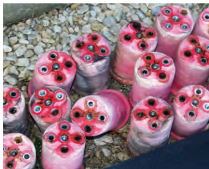
7. Glastic stand-offs used in many of the original cells were replaced with more durable Crown-sulators
