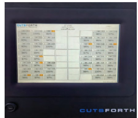
8. Cutsforth's Brush Monitoring System allows technicians to check brush wear via the display shown
