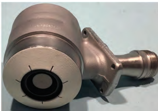
7. Post-repair flow testing and matching ensure "new" fuel nozzles with no internal cracks and within specified tolerances for optimal combustion performance
