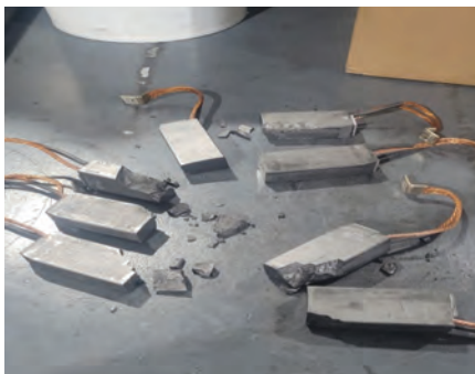
6. Generator brushes (were chipping and breaking regularly)
